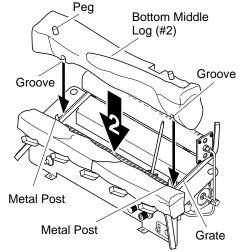
Figure 17 - Installing Bottom Middle Log (#2)
